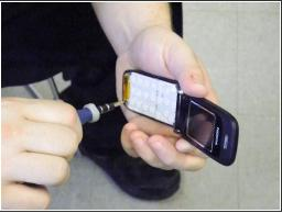
• Use a T6 screwdriver to remove the four screws (one from each corner of the keypad).
