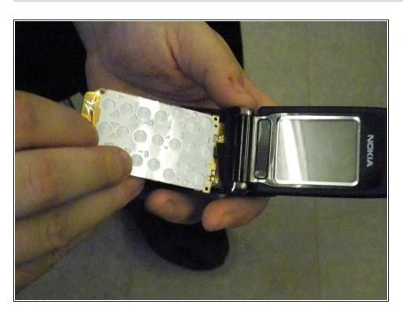
Carefully lift and remove the keypad.
