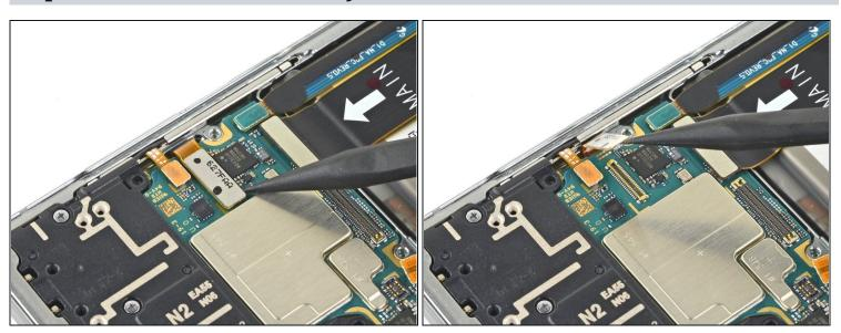
Use the pointed end of a spudger to disconnect the S-Pen touch layer cable connector from the motherboard.
