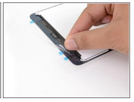
Peel and remove the clear plastic stiffening layer from all four adhesive strip sections.
