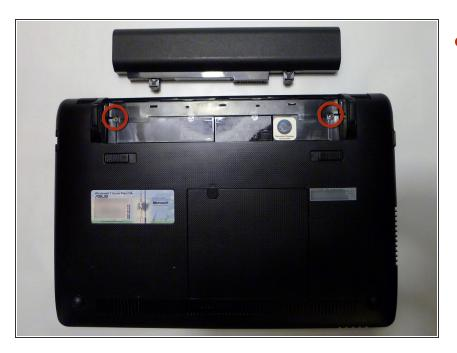
Remove screws on the battery compartment.
