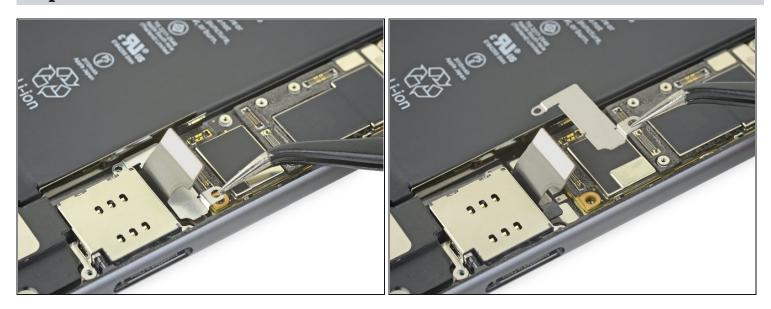
Remove the SIM reader's connector bracket.
