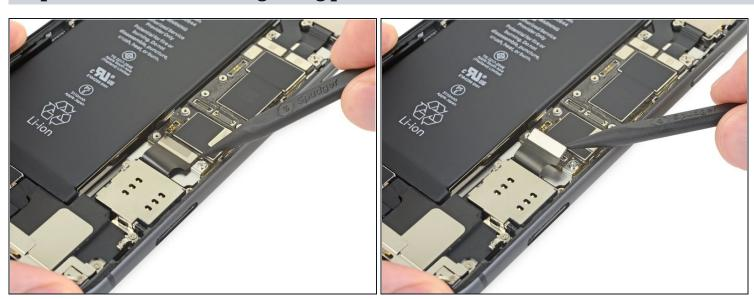
Use a spudger or a fingernail to pry up and disconnect the flex cable for the Lightning connector assembly.
