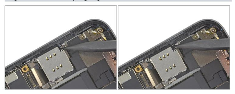
• Use the point of a spudger to push the SIM eject plunger out towards the edge of the phone.
