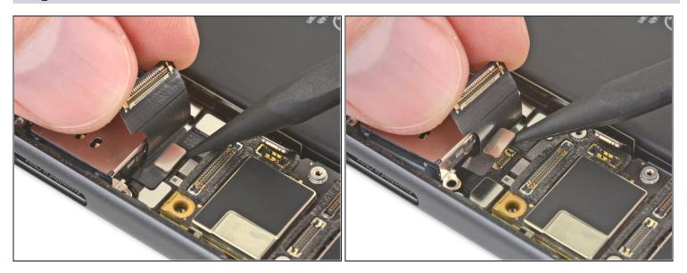
• While gently lifting the Lightning connector flex cable out of the way, use the point of a spudger to pry up and disconnect the SIM card reader flex cable.
