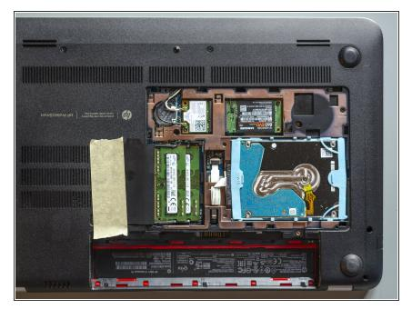
Without bending it, gently turn the RAM modules' protective flap to the left and stick it to the base enclosure with a piece of adhesive tape.
