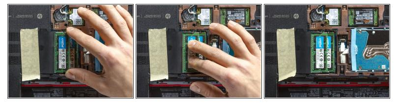
• Repeat the same process in order to insert the remaining module and it's done!
