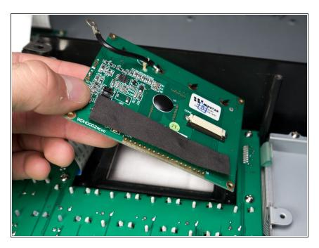
Lift the screen from either side, removing it from the board.
