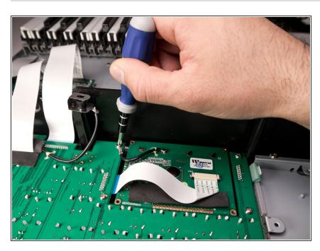
Using a Phillips #2 screwdriver, remove the one 9.8mm screw holding down the ground wire.
