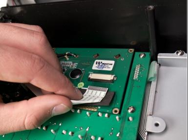
• Using two plastic opening tools, slide the black locking mechanism on the ZIF connector towards you. This will remove the ribbon cable connecting the motherboard to the screen.
