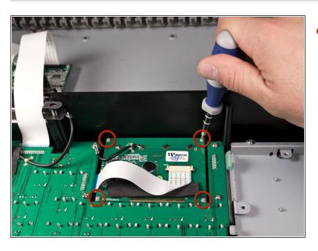
Using a Phillips #00 screwdriver, remove the four 8.9 mm screws.
