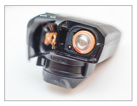
Open battery cover and remove AA battery
