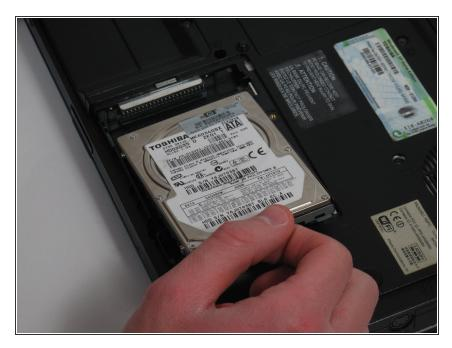
Pull the black plastic tab horizontally away from the hard drive to disconnect and remove the hard drive from the laptop.
