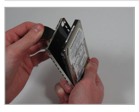
Pull the black tab away from the hard drive to separate the hard drive and the casing. To reassemble your device, follow these instructions in reverse order.
