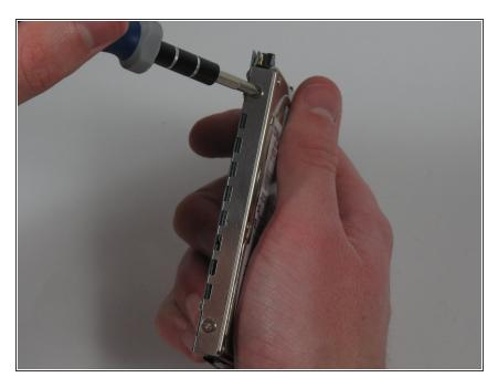
Use the Phillips 00 screwdriver to remove the four 6.50mm screws on the sides of hard drive.
