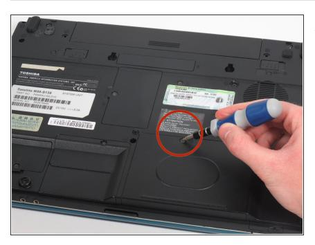
Use the Phillips 00 screwdriver to remove the 3.62mm screw.
