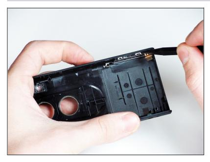
Using a spudger, carefully remove the metal casing that is attached to the ZIF connector.
