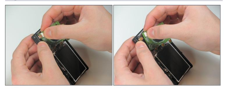
• Using your hand, or a pair of <u>tweezers</u>, remove the ZIF connector by gently pulling it out of the dock on the circuit board.
