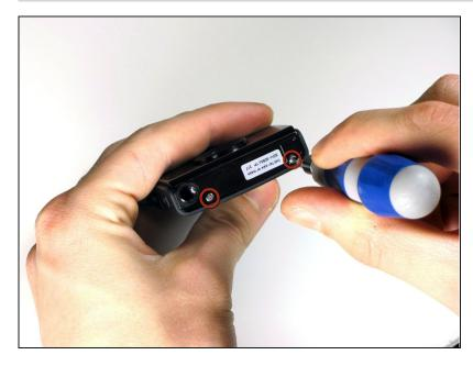
Remove the two 2.5mm Phillips #00 screws using the Philips #00 screwdriver.
