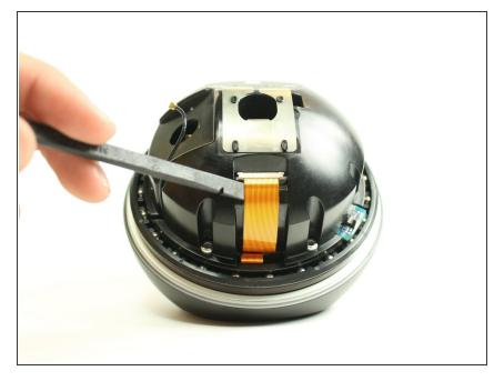
• Undo the ZIF connector by prying it with a spudger.
