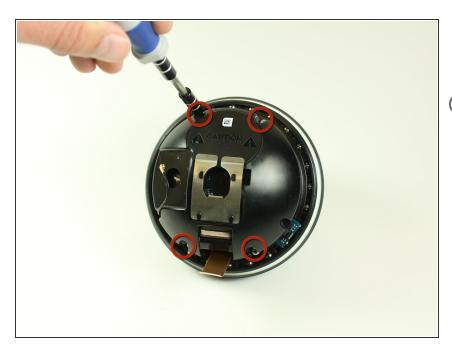
• Use a Phillips #0 screwdriver to unscrew the four 1.3 mm screws.
