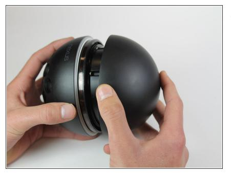
• Squeeze and pull the cap to remove it from the Nexus Q.
