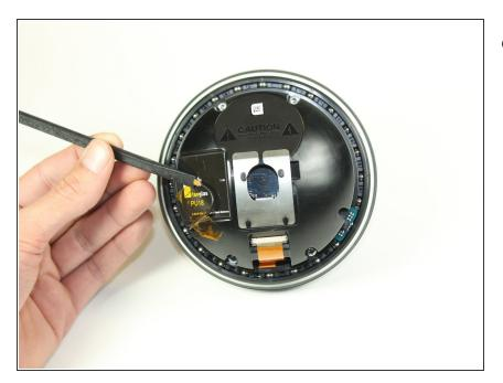
• Use a spudger to disconnect the Taoglas Wi-Fi Dual Band Antenna.
