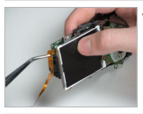
Now remove the ZIF connector from the device using a pair of tweezers.
