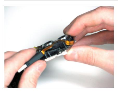
Now that the USB component is on its own, untangle the ribbon from inside the device.
