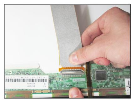
• Disconnect the video cable by pulling the grey flat wire. Now the screen is completely separate from the ThinkPad.
