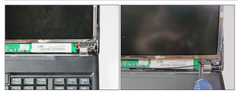
• Using a #0 Phillips screwdriver, remove the 4 mm screw.
