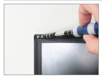
Use a #0 Phillips screwdriver to remove the eight 3.25 mm screws uncapped from the previous step.
