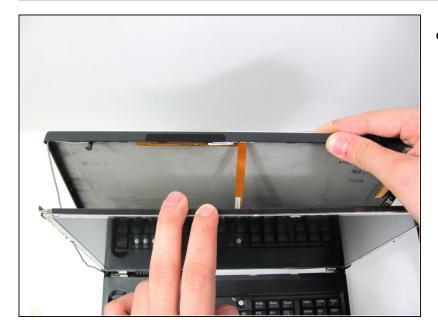
• Use your fingers to pry the screen out of its housing far enough to gain access to the ribbon cables and small screws holding the screen in place.
