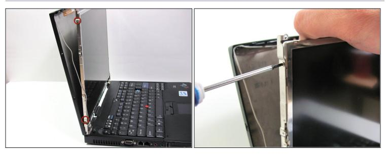
• Using a #0 Phillips screwdriver, remove the four 3.25 mm screws
