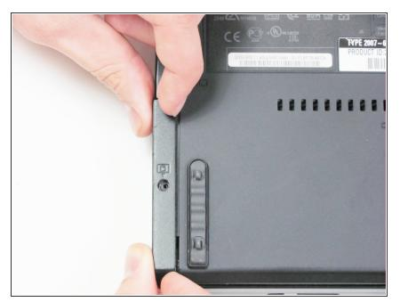
Carefully remove the plastic piece covering the hard drive port by pulling perpendicular to the side of the laptop.
