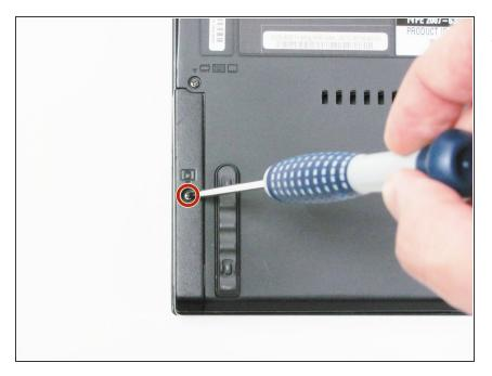
Using a #0 Phillips screwdriver, remove the 17.0 mm screw.
