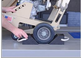
To prevent the concrete saw from rolling during service, place wheel chocks in front of and behind a rear wheel.
