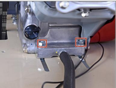
• Use a 9/16-inch wrench to loosen the five engine mounting nuts on the front and back of the engine, but do not remove them.
