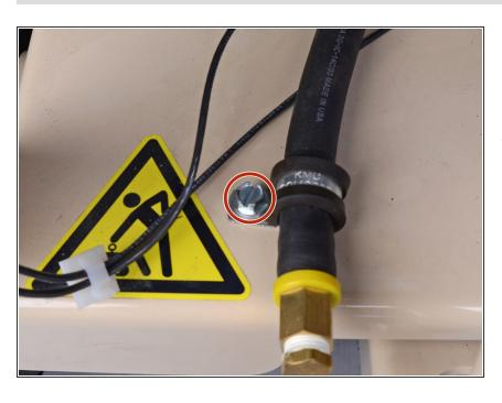
Use a flathead screwdriver or a 3/8inch wrench to remove the screw securing the drain hose to the concrete saw.
