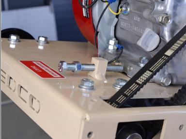
Use a 9/16-inch wrench to loosen the engine's tap bolt until the tip of the bolt is about an inch away from the engine.
