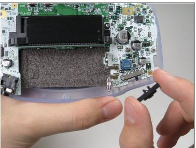
Remove the gray On/Off Switch by pulling up and away from the unit. Replace with another switch if necessary.
