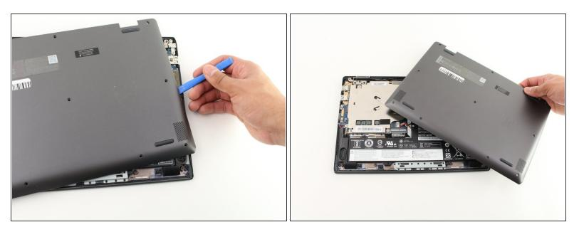
• After making sure the back panel is completely free from the body, remove the back panel.
