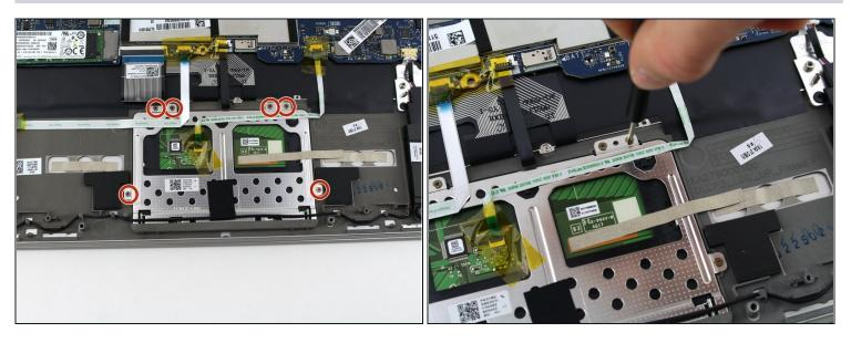
• Use a Phillips #00 screwdriver to remove the six 2.5mm screws holding down the touch pad.
