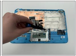
• Unscrew the three 0.2mm top screws with the Phillips #00 Screwdriver.
