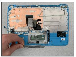
Lift up on the bracket and remove the bracket by lifting up on the metal end as shown.
