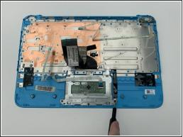
Unscrew the three 0.3mm screws holding the bottom bracket with the Phillips #00 Screwdriver.
