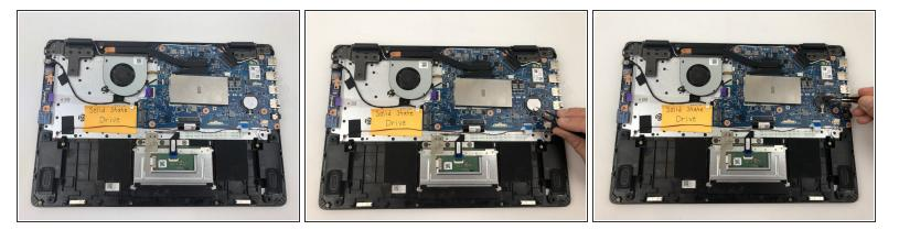
• Grasp the CMOS battery with the tweezers and remove it from the motherboard.
