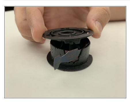
Line up the plate so that the end of the spring lines up between the teeth, and press down until the plate clicks in.
