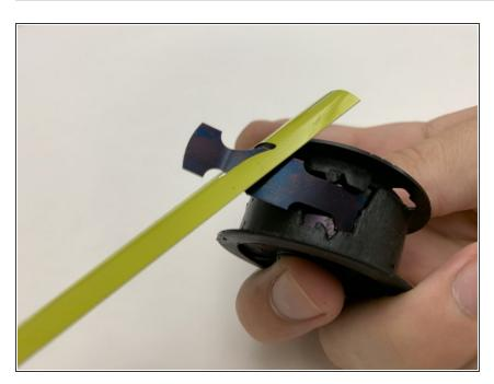
Feed the end of the spring through the hole in the tape sideways and twist the housing and tape so that the tape lines up with the slot.
