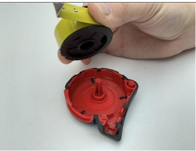
• Pull the half shell off and remove the black spring housing from the plastic axle by pulling upward.
