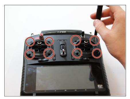
With the 5mm hex diver bit, remove the eight 10mm screws surrounding both joysticks.
