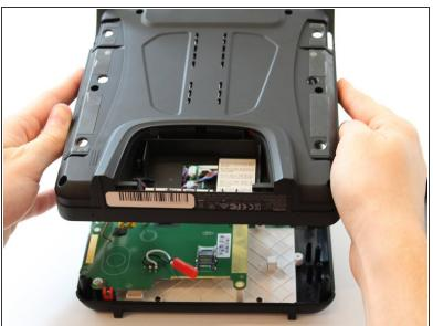
Carefully pull up and over on the back panel to remove. Take your time because there are wires connecting the two panels that can be easily torn.
