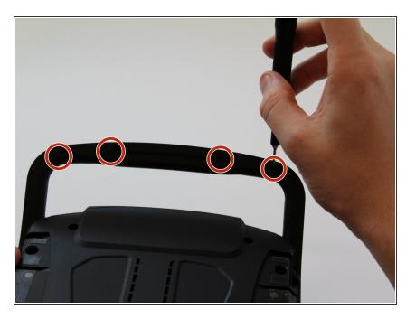
Remove the four 6mm screws from the handle using the 4mm hex driver bit.
