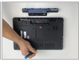
Unscrew the two 7.9mm Phillips #0 screws that secure the service cover.
