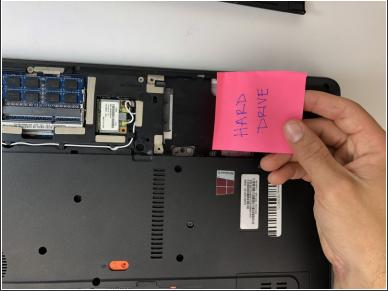
Remove the hard drive by lifting up the right side, releasing the hard drive from the compartment clips on the left. To reassemble your device, follow these instructions in reverse order.
