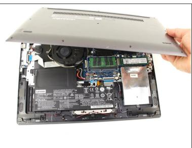
Once all the clips have been disengaged, lift off the back cover.
