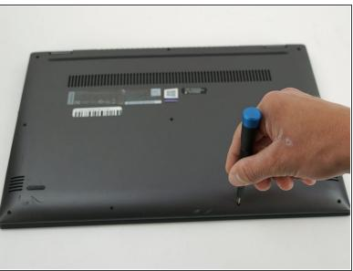
Remove the ten 5 mm Phillips #00 screws that are holding the back panel on.
