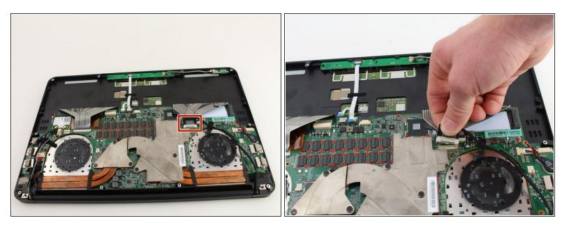
Remove the cable connecting the motherboard to the display by gently puling it upwards with your fingers.
