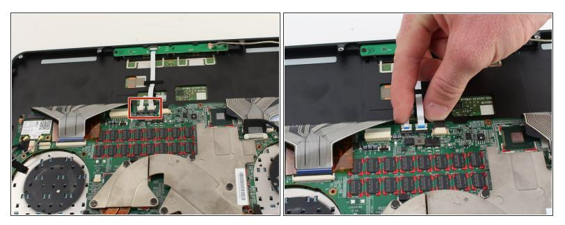
• Remove the small connectors connecting the motherboard to the trackpad by first flipping up the plastic crimps and then pulling them away from the motherboard with your fingers.
