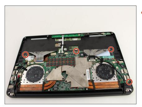
Using the Phillips #0 screwdriver, remove the four 3mm screws connecting the motherboard to the chassis of the device.
