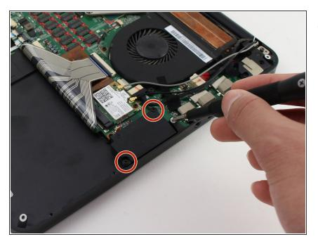
Using the Phillips #0 screwdriver, remove the two 3mm screws from the right speaker.
