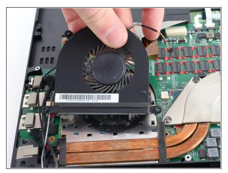
Holding the rounded edge of the fan, slowly lift upwards until it is removed.
