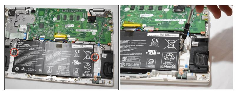
Remove two 4.6 mm JIS # screws at each end of the battery.
