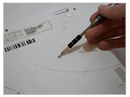
Remove eleven 7.2 mm screws from the bottom of the Chromebook using a JIS #1 screwdriver.
