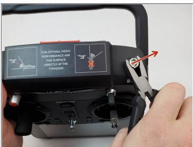
Twist counter clockwise on the silver portion of the device with a pair of pliers.
