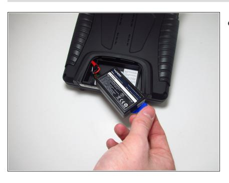
Gently lift the blue tab connected to the battery in order to remove the battery from its housing.
