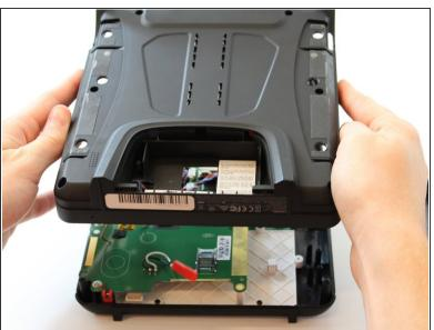
Carefully pull up and over on the back panel to remove. Take your time because there are wires connecting the two panels that can easily torn.
