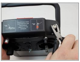
Grab ahold of the top of the black cap on the button with the pliers and pull up forcefully.
