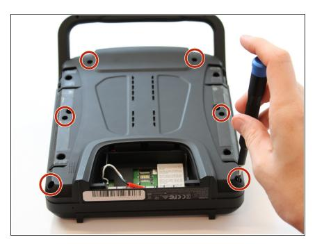
Remove the six 1.3 cm screws located on the back panel of the remote using the 5.5mm hex screw bit.
