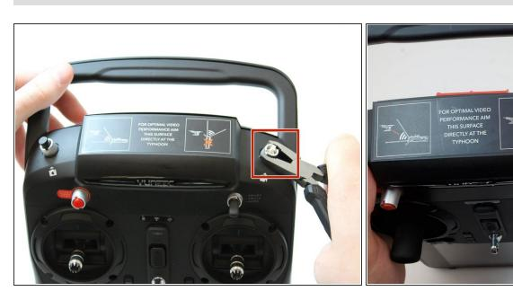
Twist counter clockwise on the silver portion of the device with a pair of pliers.
