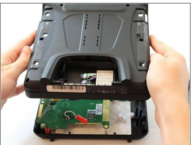
Carefully pull up and over on the back panel to remove. Take your time because there are wires connecting the two panels that can easily torn.
