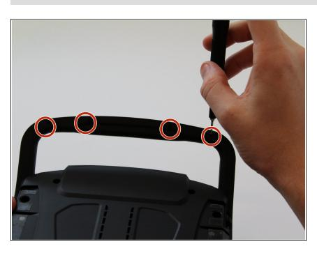
Remove the four 6mm screws from the handle using the 4mm hex driver bit.
