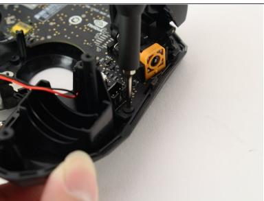
Remove the two T6 Torx screws.
