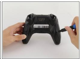
Remove the six T6 Torx screws from the back of the controller.
