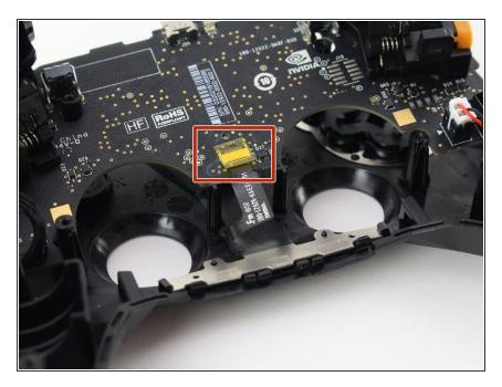
Remove the yellow plug from its socket.
