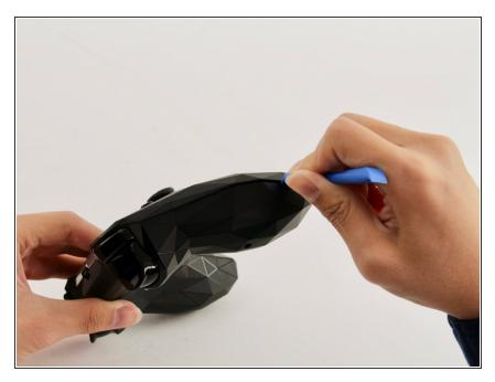
Gently open the top frame of the cover with the plastic opening tool.
