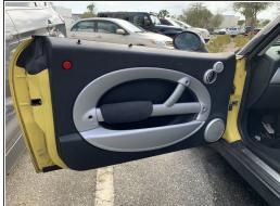
Snap on the handle and speaker cover using your hand. And once, again, use enough pressure to snap it back in place, and not excess pressure.
