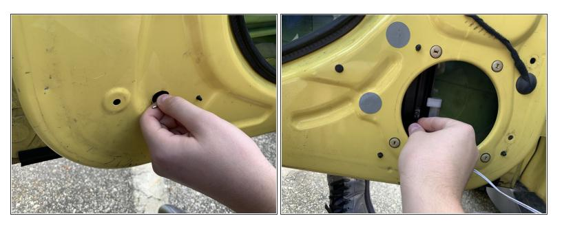
Roll down the window all the way again and replace the two screws in the bottom-left corner and speaker hole with the 5/32 Allen key to secure the window rollers.
