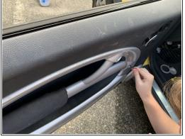
Using the Phillips #3 Screwdriver, screw in the three side panel screws back into place.
