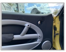
Remove the handle and speaker cover using a flathead screwdriver.
