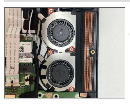
Remove the four remaining screws located on the fan using the Phillips #00 screwdriver.
