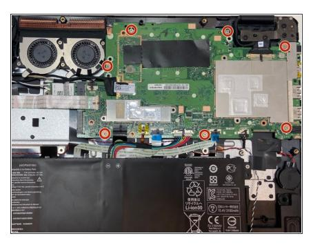
Remove seven 3 mm screws using the Phillips #00 screwdriver.
