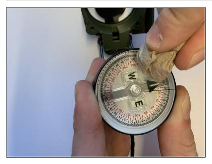
• Using small circular motions clean the inner lens.
