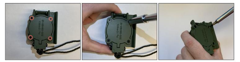
• Using a Phillips #1 screwdriver, remove the four screws in the bottom of the compass.
