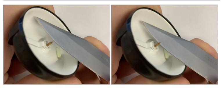
$\triangle$  Use the edge of the pocket knife to sharpen the needle upwards.
