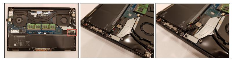
A Before proceeding, be sure to disconnect the battery. Failure to do so may cause damage to the device.
