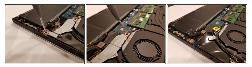
Use a Phillips #00 screwdriver to remove the two screws holding down the the display cable fastener.
