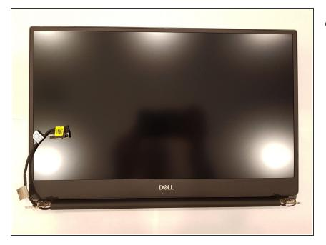
Pull the display assembly away from the rest of the case.
