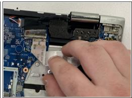
• Use the Reverse Tweezers to remove the ribbon wires connecting the speaker to the motherboard.
