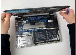
Using the opening tool, carefully remove the bottom cover from the device.
