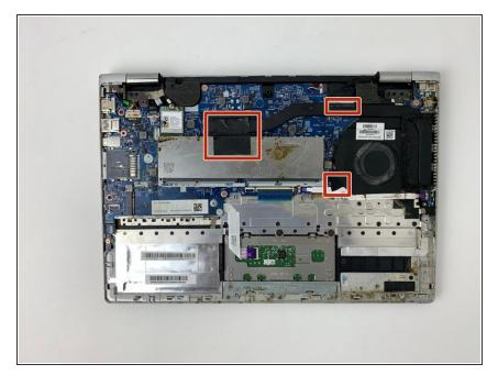
Remove the tape that secures the fan to the computer.
