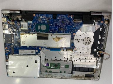
Flip the device over so the hinge is at the top and the motherboard, and other components are visible.
