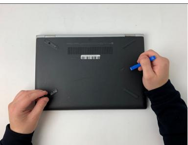
Use the opening tool to remove the rubber feet attached to the bottom of the device.
