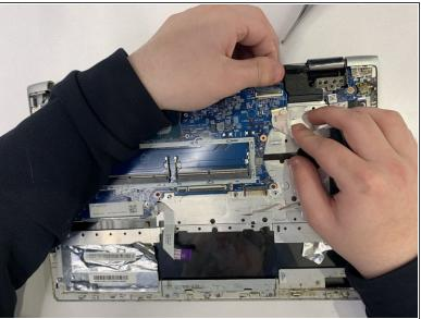
Grab the ribbon wires by the edge of the socket and pull to remove them from the motherboard.
