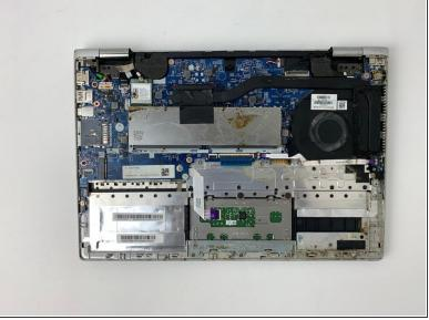
Carefully lift from the base and remove the battery.
