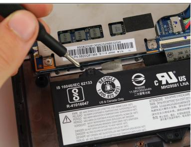
• Remove the five 3.9 mm Phillips #00 black screws holding the battery in place.
