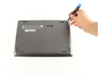
Remove the ten screws with a Phillips #00 screwdriver.
