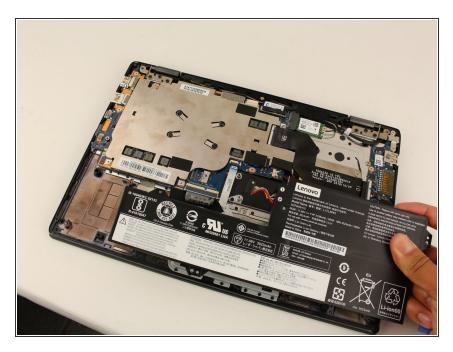
Remove the now disconnected battery from the laptop.
