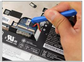
• Pull out the multicolored connecting cables using an iFixit opening tool.
