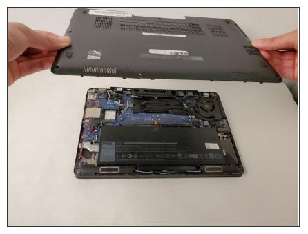
• Lift and remove the panel.
