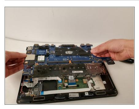
Lift and remove the motherboard by grabbing the outside edges and pulling straight up.
