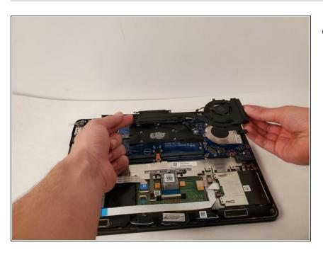
Lift and remove fan by pulling gently straight up using your fingers
