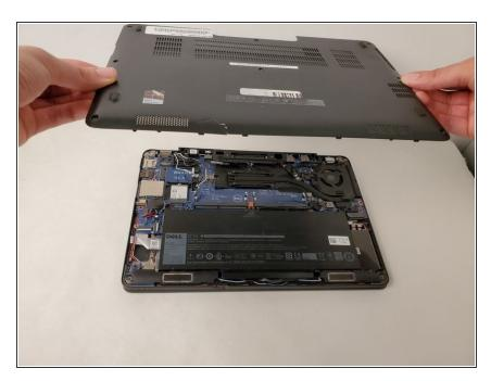
Lift and remove the panel.
