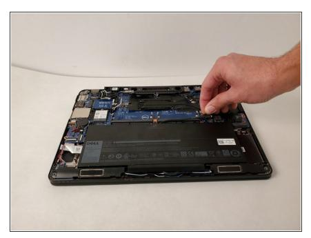
Disconnect the battery wire by using your fingers to pull diagonally left on the tab.
