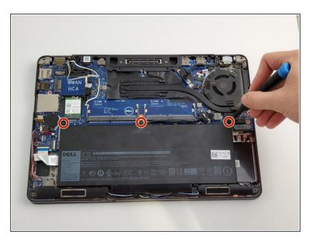
Remove the three M2.5 X 5MM screws, located above the battery, with a Phillips #00 screwdriver.
