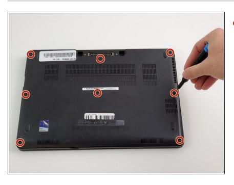
Remove all eight M2.5 X 8MM screws with a Phillips #00 screwdriver.
