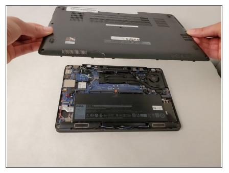
• Lift and remove the panel.
