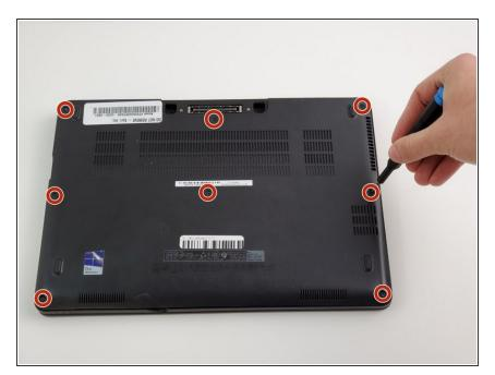
Remove all eight M2.5 X 8MM screws with a Phillips #00 screwdriver.
