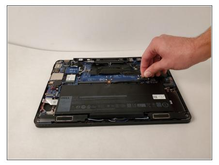
Disconnect the battery wire by using your fingers to pull diagonally left on the tab.
