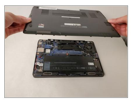
Lift and remove the panel.
