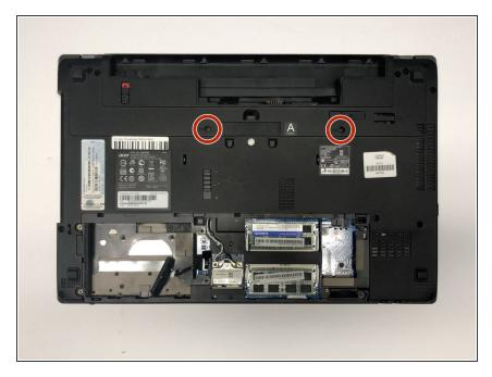
Remove the two 7mm Phillips #1 screws.
