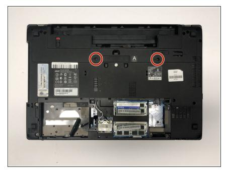
Remove the two 7mm Phillips #1 screws.
