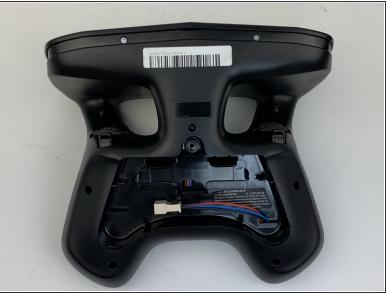
Remove the battery from its brackets by pulling up on the ends of the battery.
