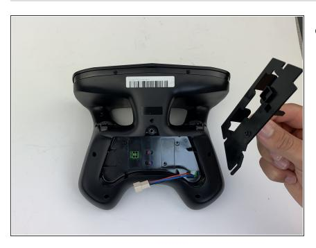
Remove the battery compartment plate by pulling up and out.
