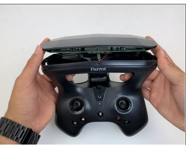
Remove the top plate by pushing on the corners with your hand.
