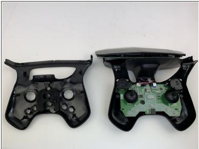
Remove the face plate by pulling up and out.
