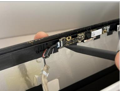
Using the spudger, carefully remove the webcam connector from the metal frame.
