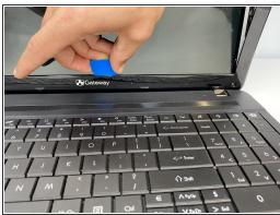
Using the opening pick in between the front cover and bezel, gently loosen and lift the plastic bezel from the screen and backing.
