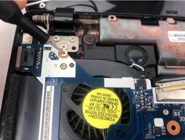
• Use the Phillips #000 driver to remove the two remaining 3mm silver screws.
