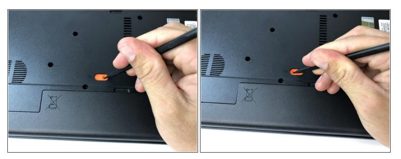
Using the spudger, push the orange tab to the unlock position.
