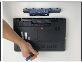
Unscrew the two 7.9mm Phillips #0 screws that secure the service cover.
