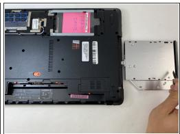
Using the flat end of the spudger, slide the optical drive out.
