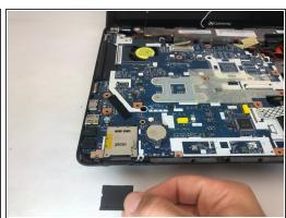
Use the spudger to slide the SD card out of the back left corner of the system board.
