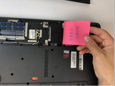
Remove the hard drive by lifting up the right side, releasing the hard drive from the compartment clips on the left.
