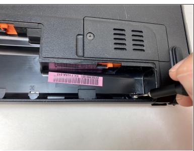
Using a Phillips #000 driver, remove the three silver 0.79mm screws located on the back edge of the battery compartment.
