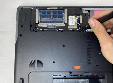
Using a Phillips #000 driver, remove all nineteen of the remaining 0.79mm screws that are holding the back case in place.
