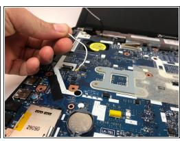
Remove the tape holding the white wire and gently pull it out of its hole.
