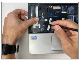
Using the spudger, gently slide the clamp holding the MS cable upward towards the screen.
