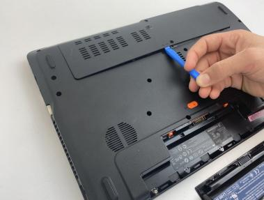
• Use the opening tool to gently pry open the compartment covering.
