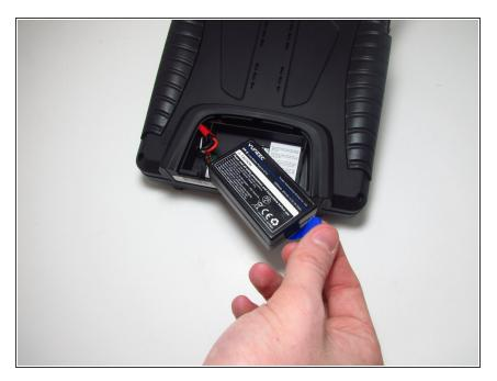
• Gently lift the blue tab connected to the battery in order to remove the battery from its housing.
