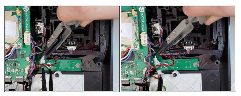
• Using the tweezers, disconnect your screen connection wires.
