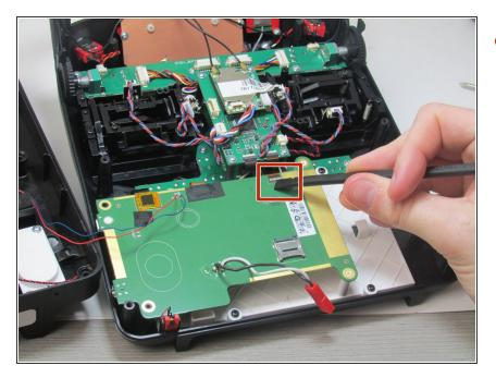
Take the flat end of the spudger and place it under the white lock on the ribbon cable's ZIF connector. Then lift it up on the white lock to allow the ribbon cable to be removed.
