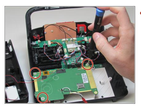
Take a Phillips #0 screwdriver to unscrew the three 5mm screws on the screen circuit board.
