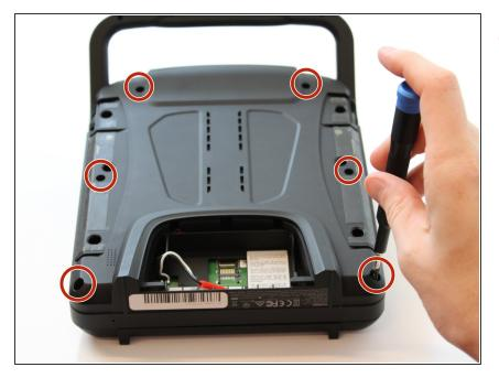
Remove the six 1.3 cm screws located on the back panel of the remote using the 5.5mm hex screw bit.
