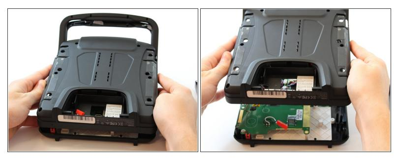
• Carefully pull up and over on the back panel to remove. Take your time because there are wires connecting the two panels that can easily be torn.
