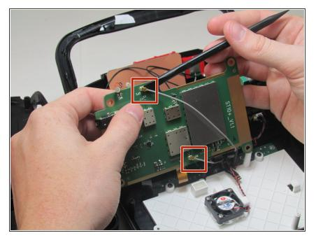
Carefully disconnect the two wires connected underneath the screen motherboard with the plastic spudger.
