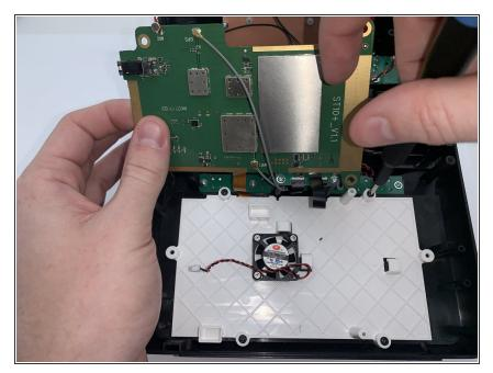
• Using the Phillips #0 screw driver, remove the four 6mm screws holding the screen fan plate on.
