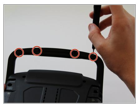
Remove the four 6mm screws from the handle using the 4mm hex driver bit.
