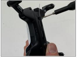
Using a Phillips #00 Screwdriver remove the eight 4mm screws on the bottom of the drone.
