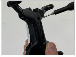
Using a Phillips #00 Screwdriver remove the eight 4mm screws on the bottom of the drone.
