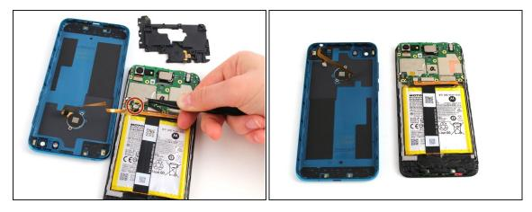
Use the angled tweezers to pry off the metal head of the connecting piece from the main motherboard assembly.
