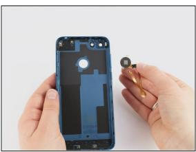
• Use the angled tweezers to pull up on the two tabs connecting the scanner to the back plastic panel, and disconnect the fingerprint scanner from the back of the device.
