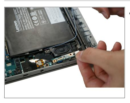
Remove the circuit board by hand.
