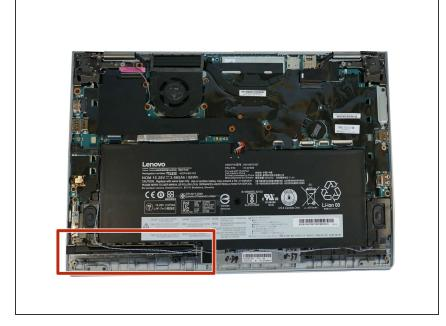
Remove the pen from its slot on the side of the laptop before removing the pen charging port.
