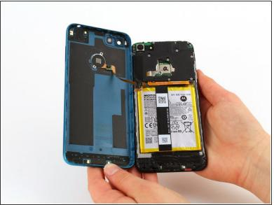
Run the halberd spudger along the edges of the device. The back cover should easily pop off.
